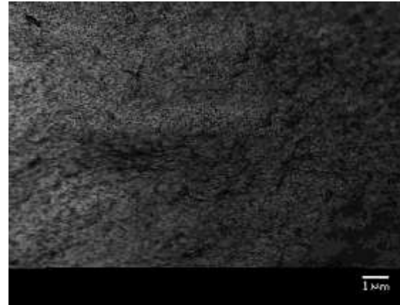
(a) (b) Fig. No. 5 –SEM images of untreated (a) and corona treated (b) LDPE films
